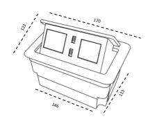
**Panel size**: 170 x 123 mm /2.5 mm **Base box size**: 146 x 113 x 95 mm
