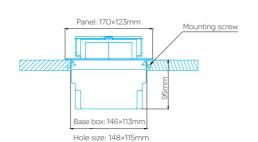
**Panel size**: 170 x 123 mm /2.5 mm **Base box size**: 146 x 113 x 95 mm
