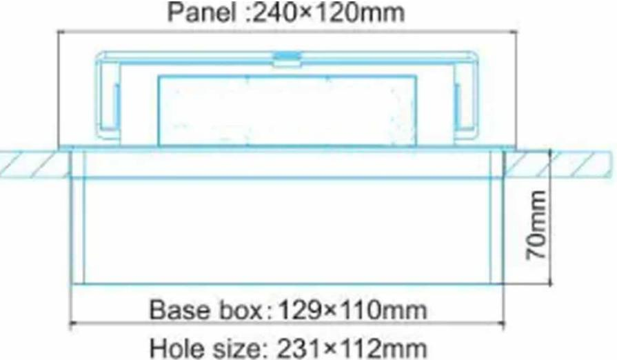
(reverse) can lead multi-str& wire cable out of the floor socket & effectively protect the wire cable skin against damaging.
